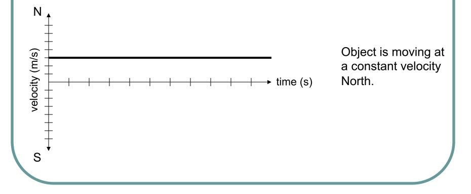
A horizontal line on the V-T graph means constant velocity.
