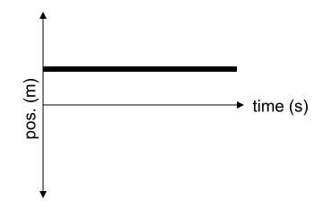
A horizontal segment means the object is at rest.
