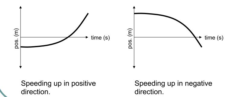
Curved segments on the D-T graph mean the object's speed is changing.
