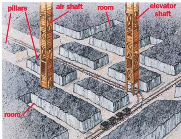
Most mines used a room-and-pillar method for extracting coal. This entailed digging out "rooms" of coal off a series of tunnels, leaving enough coal behind to form a pillar that prevented the room from collapsing.
